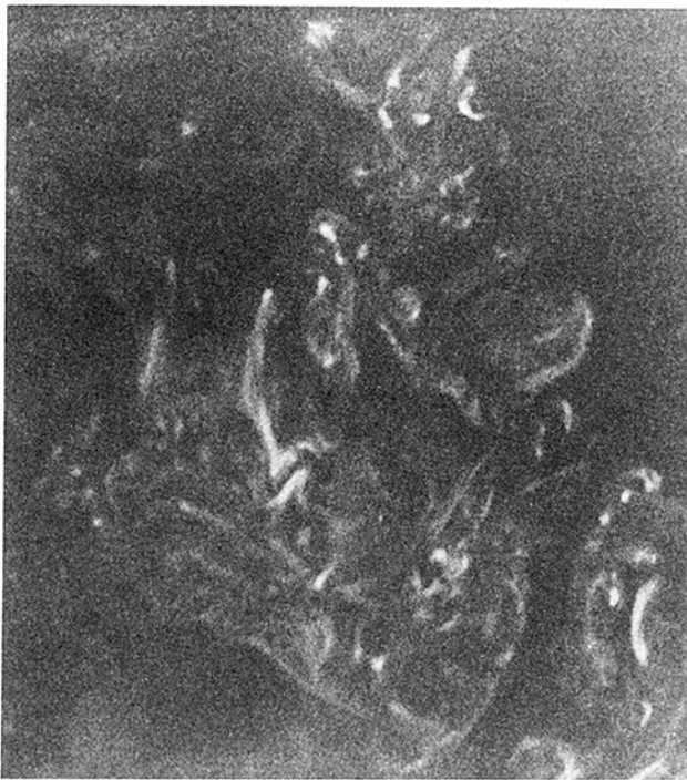
Fig. 5 Light-sheet photograph of soot particles in an acetylene/air diffusion flame: Re = 5300
